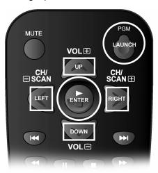
PGM key launches PROGRAM MODE LEFT and RIGHT keys NAVIGATE UP and DOWN keys CHANGE VALUES CENTER key
